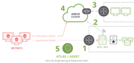
Figure 1: The fully integrated combination of 1) AED/APS on-premise to stop application layer attacks; 2) Cloud Signaling to intelligently reroute large attack to Arbor Cloud; 3) Cloud-based flow collection, attack detection and reroute to Arbor Cloud; 4) Multi-Tbps of Arbor Cloud global scrubbing; 5) All continuously armed with the global threat intelligence of ATLAS/ASERT - offers the most comprehensive DDoS protection solution in the industry.
